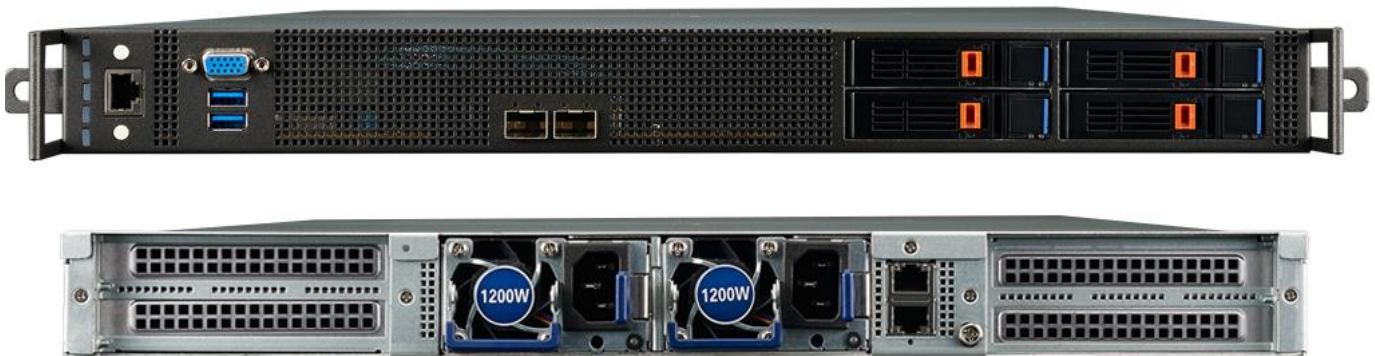
Figure 7: Advantech SKY-8101D front and rear views
