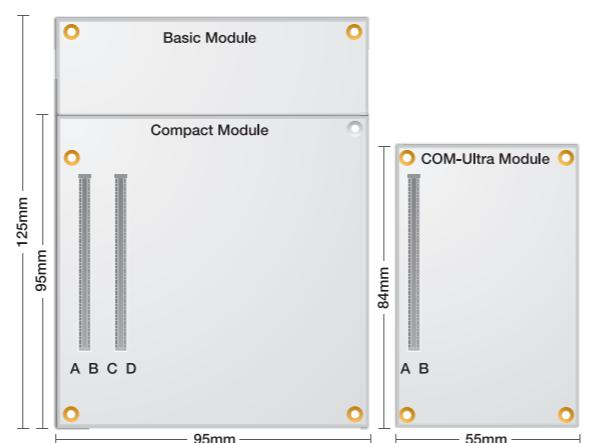
Even though the Compact Module size is already known in the market it is now also officially supported in the standard specification. The Compact Module form factor allows designs with up to 2 B2B connectors thus all existing pin out definitions can be realized on the module.
